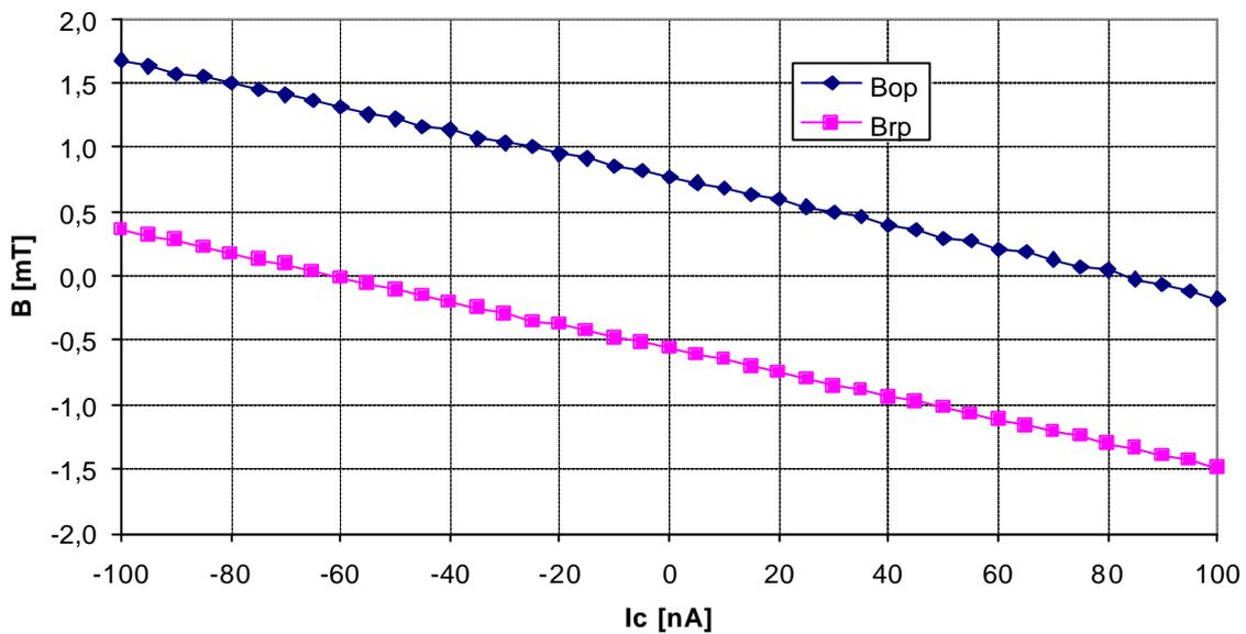
**TLE4921-3U: Threshold shift vs. filter leakage current  $I_c$
